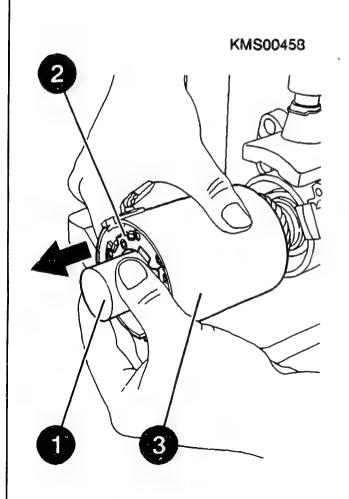
Disassembling drive-end bearing
